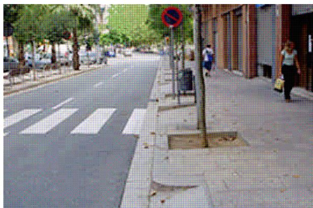
**RACCORDI PER MARCIAPIEDI E PICCOLI DISLIVELLI****1.2****SCIVOLO RETTILINEO CON RAMPA A PIANO INCLINATO E RACCORDI TRIANGOLARI.**
