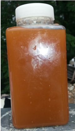
Contaminated iron (hydr)oxydes removed with air pulses into water flow
